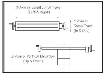
Figure 19. The directions of table movement.
